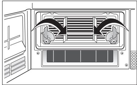
5. Use the handle to pull the heat exchanger out of the base and carry it horizontally to prevent any remaining water from spilling.
